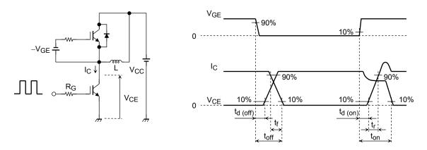
Note 2: Switching loss measurement waveforms
